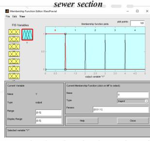
A fragment of the knowledge base for determining the categorization of a section of the sewer network
